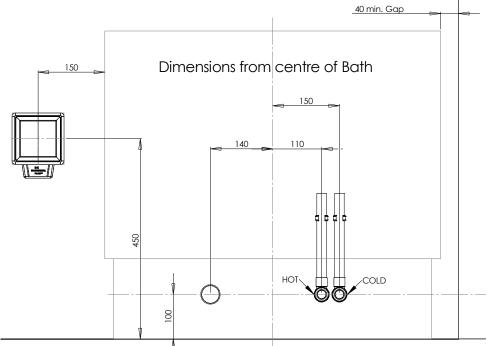
**Electrics** 230 volt, 1.25 kW WATERPROOF switched flex outlet, located in the position shown supplied by a protected fused spur.
