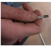
Image 5: Insert the double air hose in the new handset.
