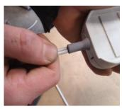
Check the proper function of the buttons. If the functions are reversed, pull the double air hose out of the handset, turn the cable 180° and reinsert.
